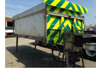
**Issues:** Hoppers have limited capacity, no unload capabilities, high center.
